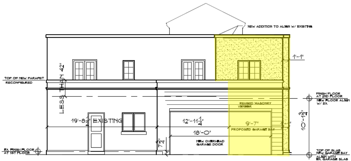
Figure 5 – Amended Corner Elevation (North)
