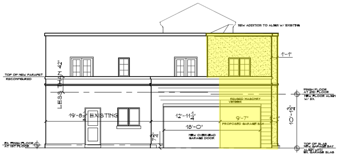
Figure 5 – Amended Corner Elevation (North)
