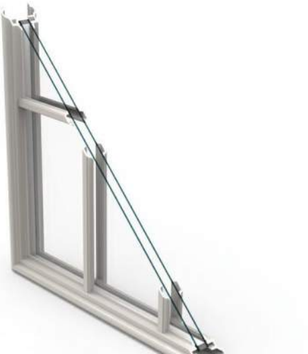
NEW IGU WITH SIMULATED DIVIDED LINES, TO MATCH EXISTING
