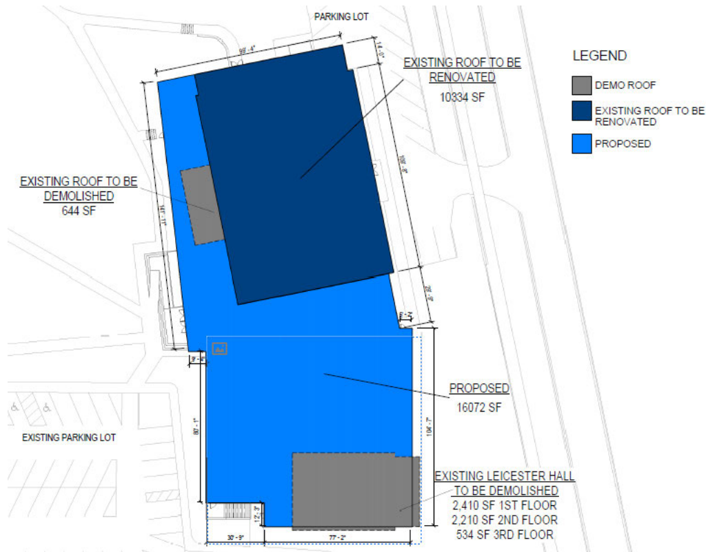
Figure 7 – Proposed Demolition and Proposed Building Footprint
