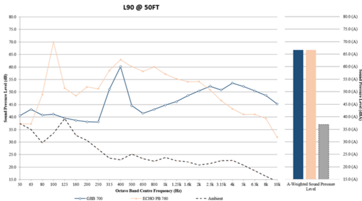
Figure 8: Audio demonstration 1 – equivalent gas and battery leaf blowers at 50 feet
