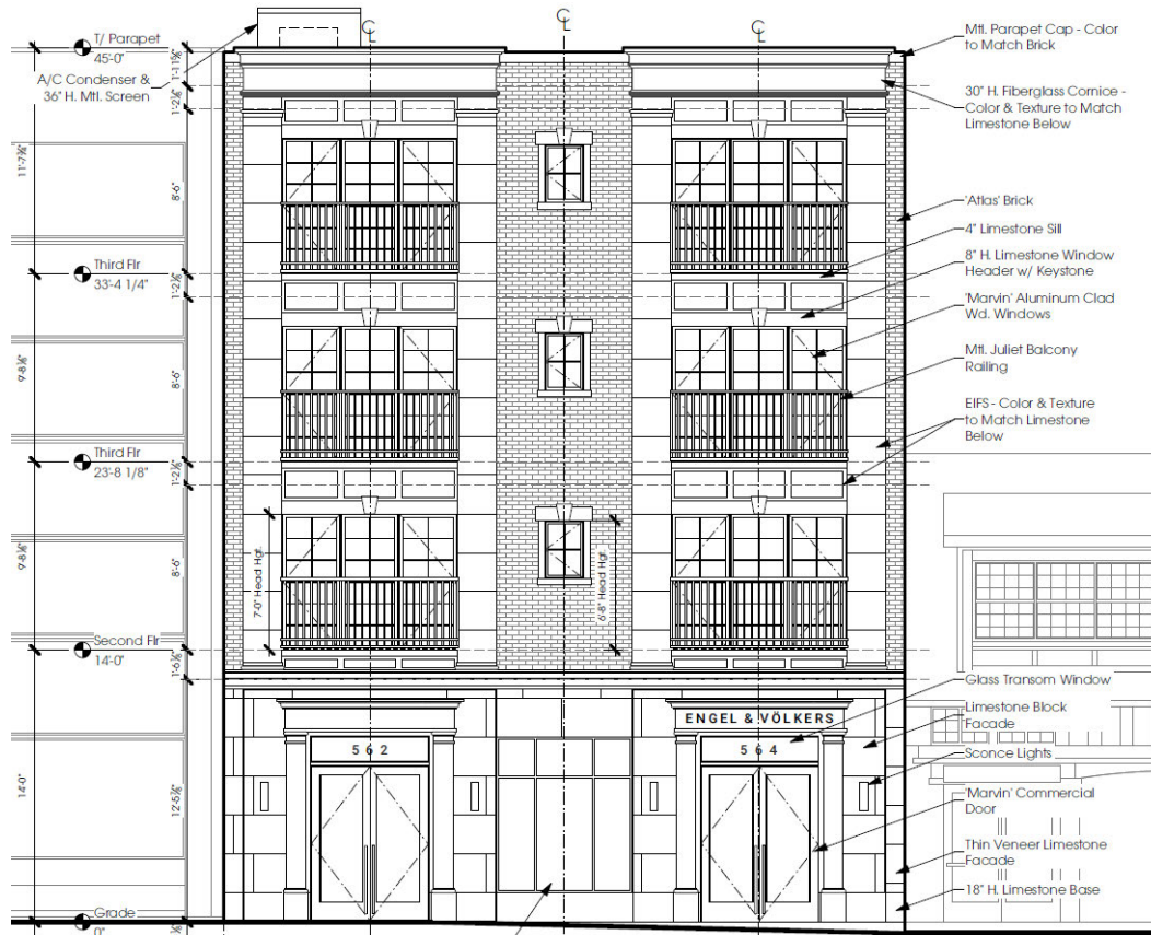
Figure 7 – Front Building Elevation – Green Bay Road
