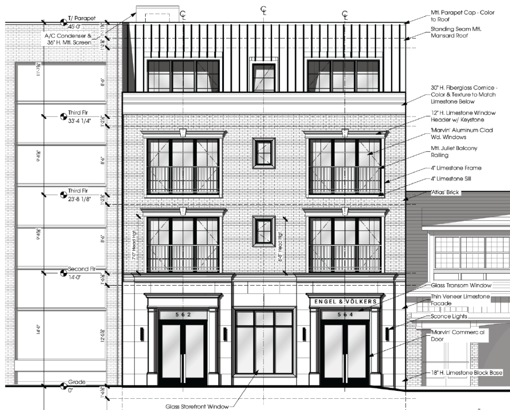
Figure 2 – Amended Front Building Elevation – Green Bay Road
