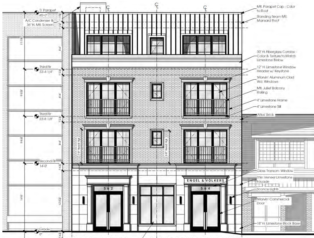
Figure 12 – Front Building Elevation – Green Bay Road
