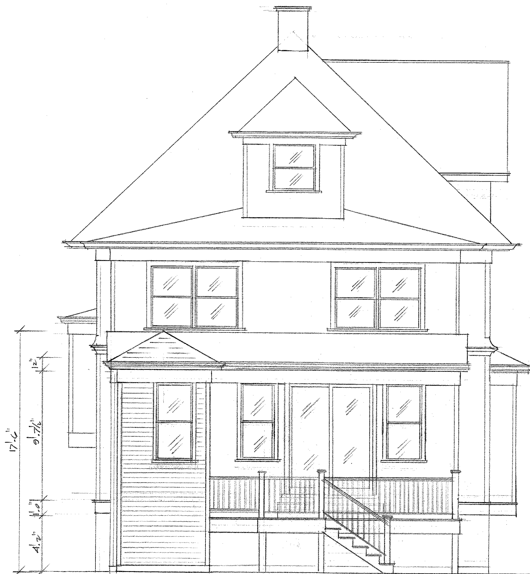
PROPOSED WEST ELEVATION 1/4" = 1'-0"
