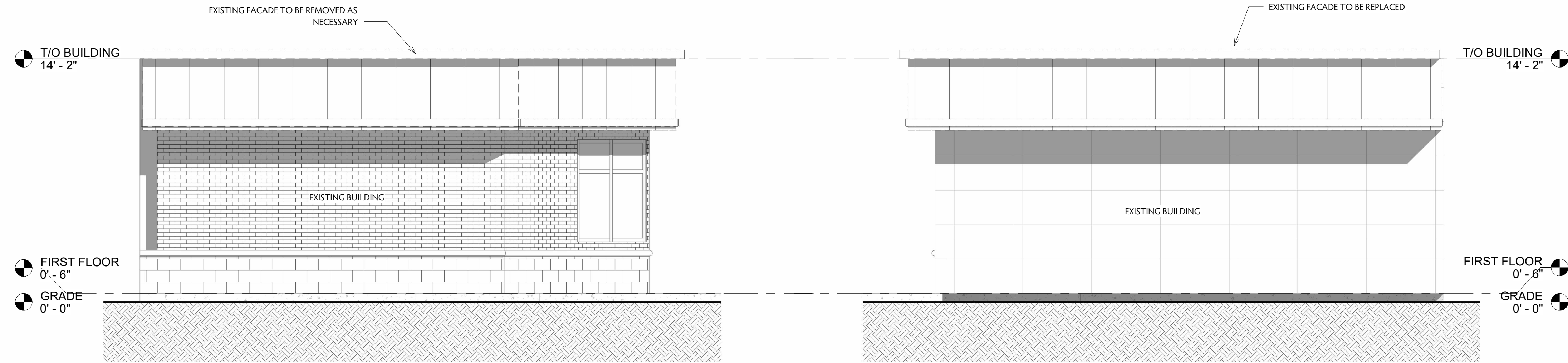
3 DEMO - WEST ELEVATION 1/4" = 1'-0"
