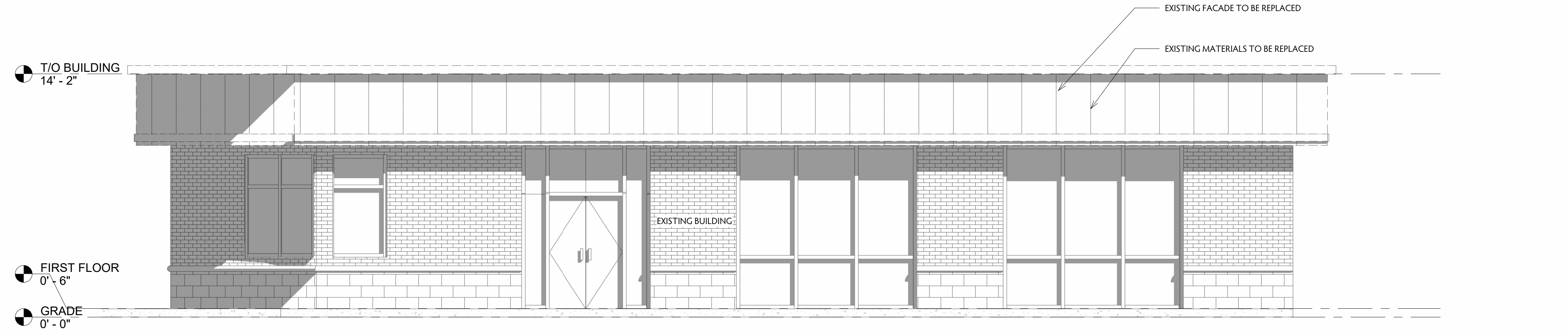
1 DEMO - SOUTH ELEVATION 1/4" = 1'-0"
