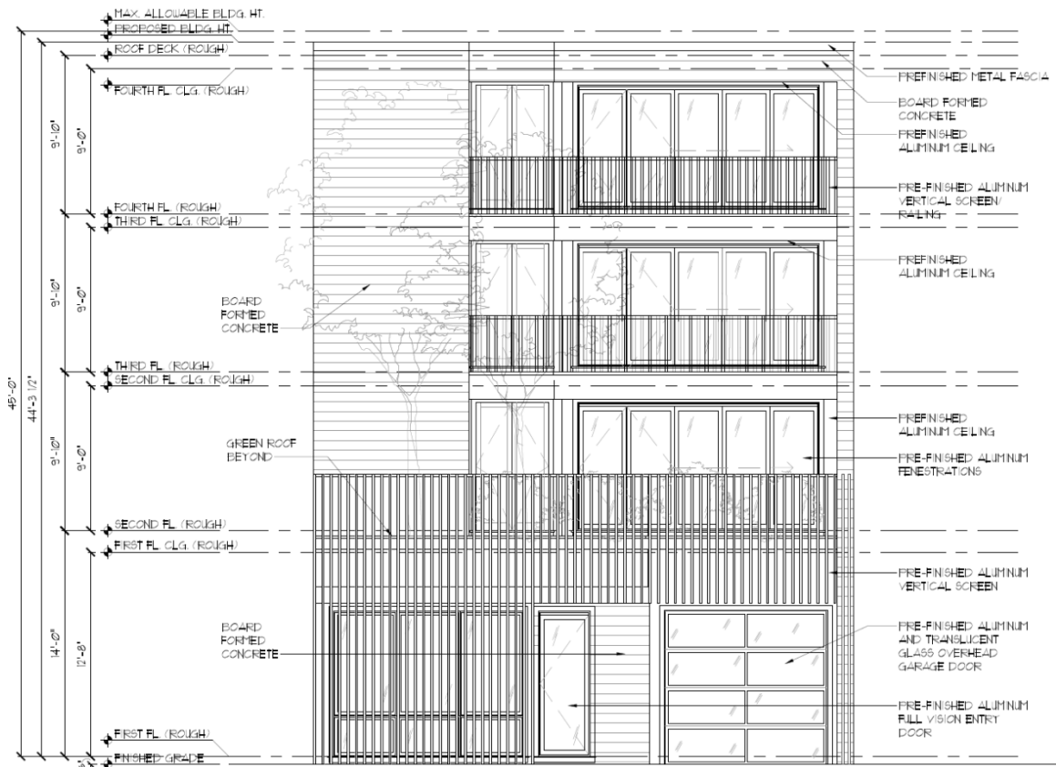
Figure 13 – Front Building Elevation – Oak Street
