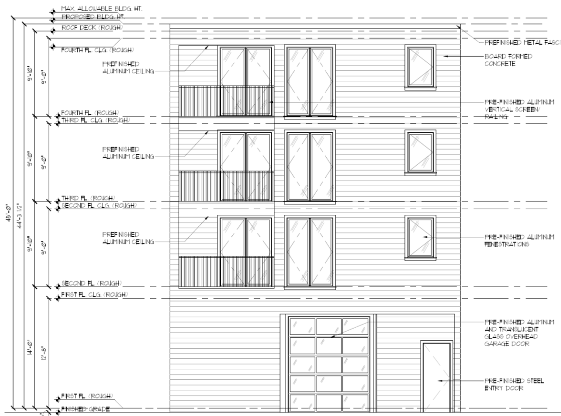
Figure 14 – Rear Building Elevation – Private Alley
