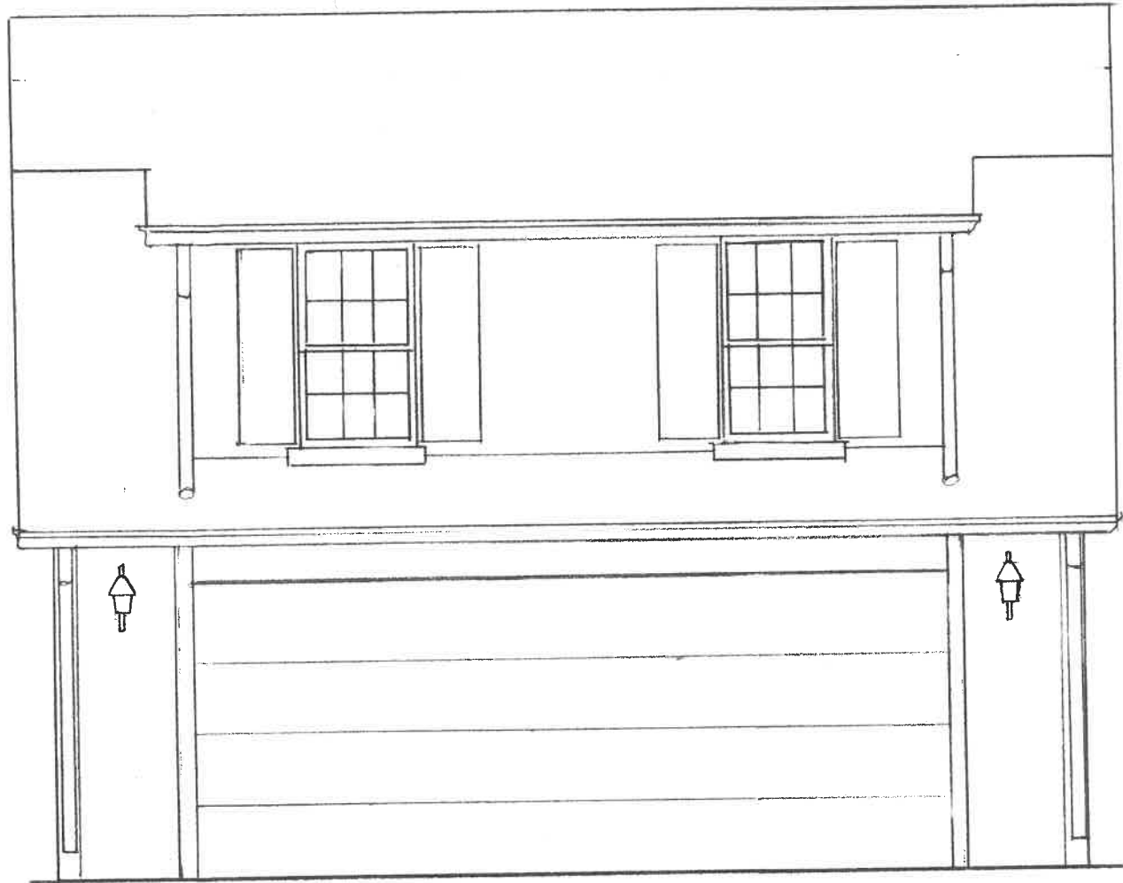
4 EXISTING N. ELEVATION W/ NEW DOOR A-1 1/4" = 1'-0"
