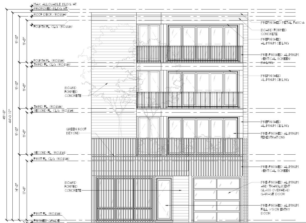
Figure 14 – Front Building Elevation – Oak Street
