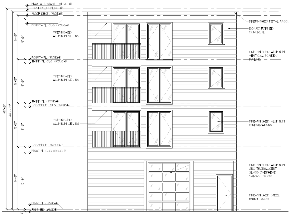
Figure 15 – Rear Building Elevation – Private Alley
