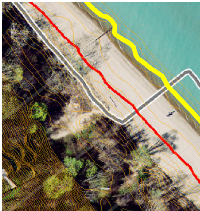
Figure 3 - 50' Setback Falls Short of Steep Slope Zone
