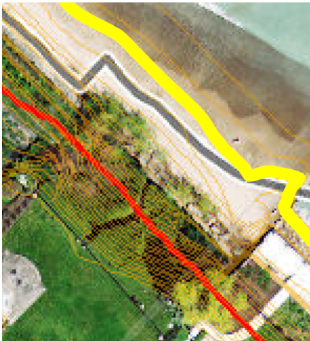
Figure 2 Setback Line Falls within Steep Slope Zone
