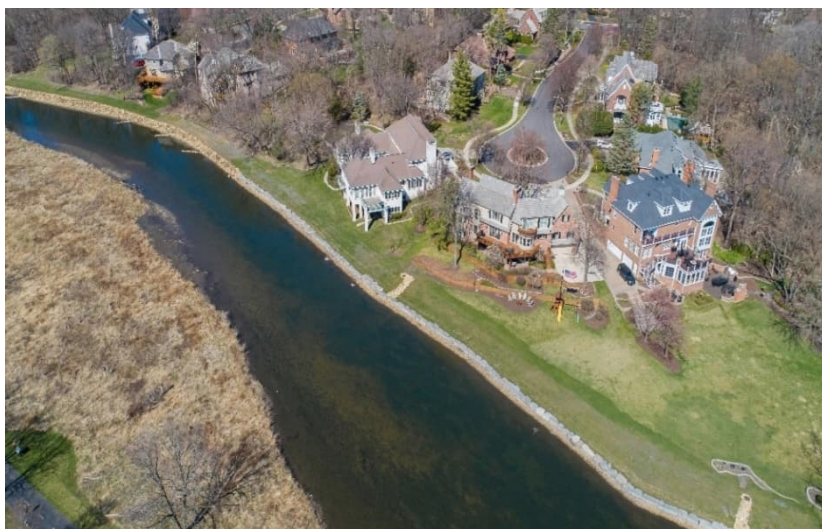
The overall project corridor showing ledge stone and vegetated boulder revetment treatment.
