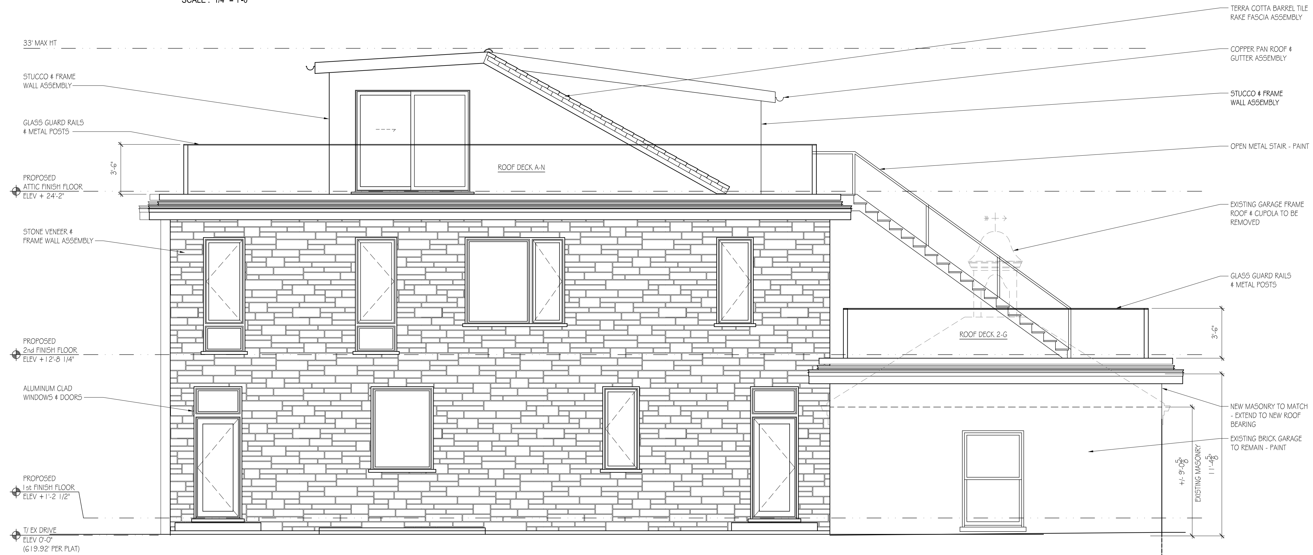
PROPOSED NORTH ELEVATION SCALE: 1/4" = 1'-0"
