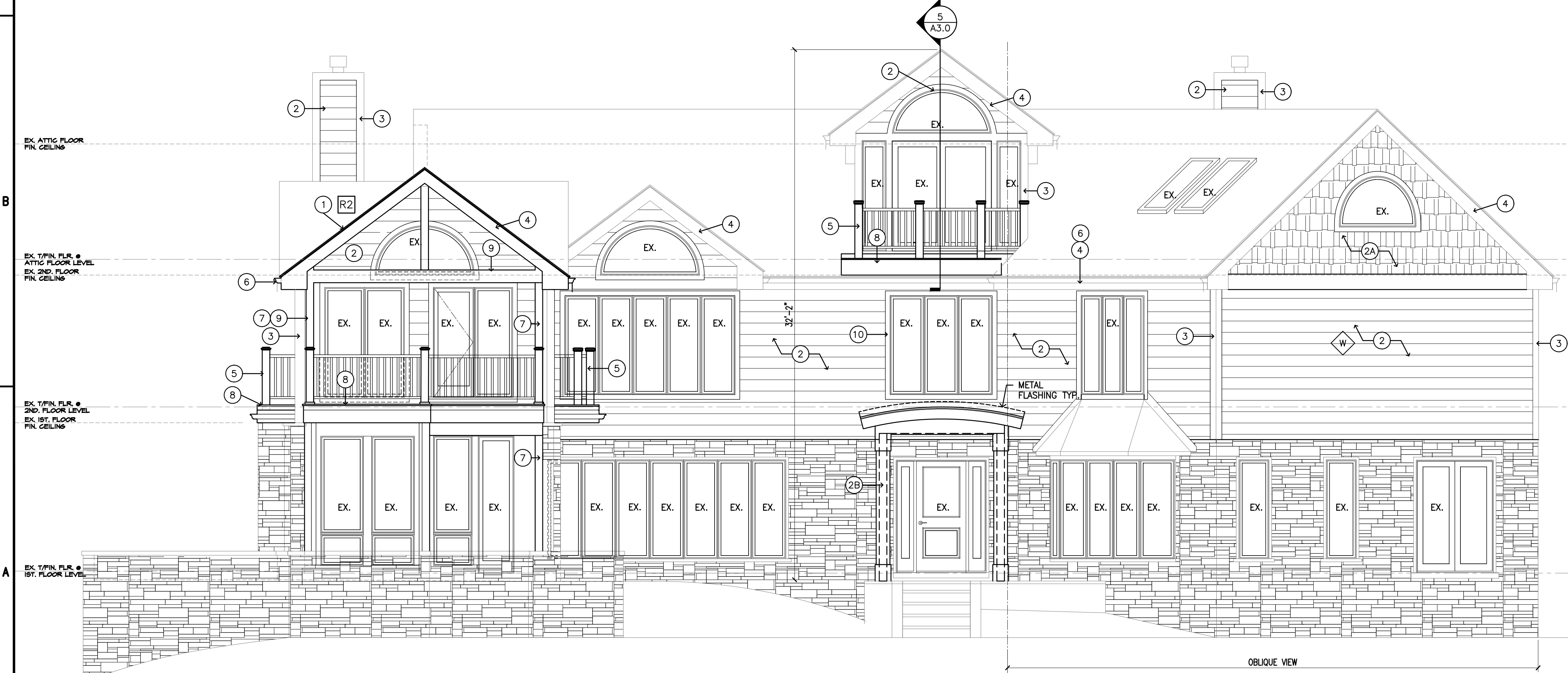
2 NEW NORTH ELEVATION 1/4" = 1'-0"
