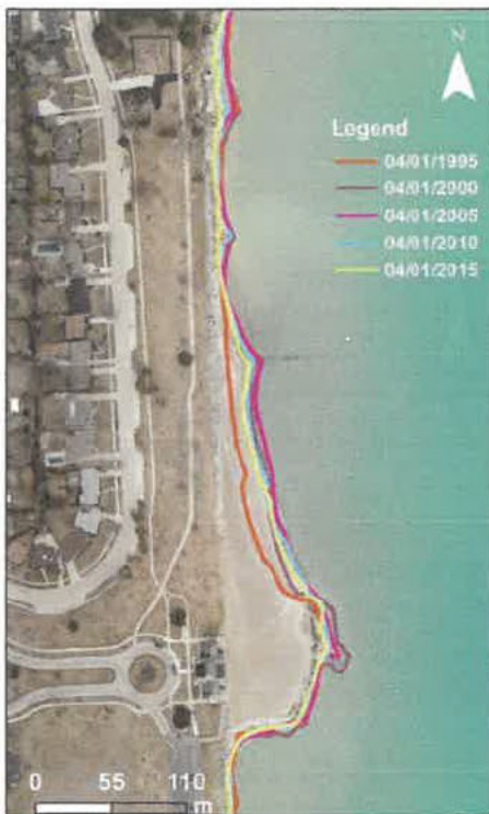
Figure 24. Shoreline position at Southport Park from 1995-2015.
