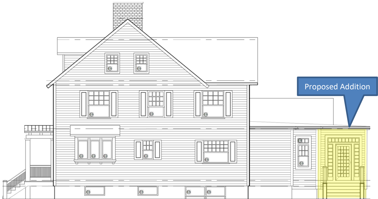
Figure 8 – Proposed Corner Elevation (Summit Street)
