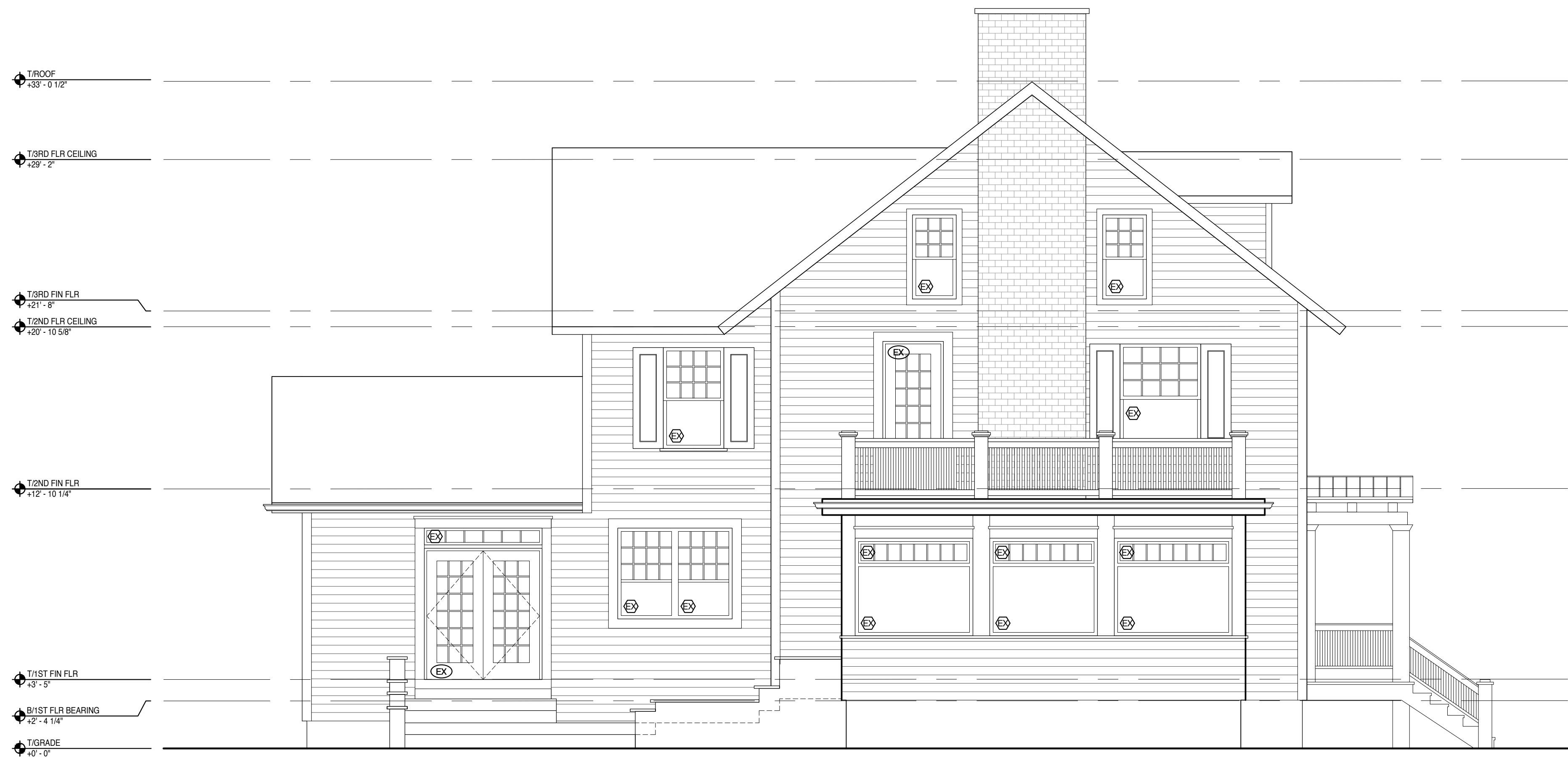
2 Existing East Exterior Elevation 1/4" = 1'-0"
