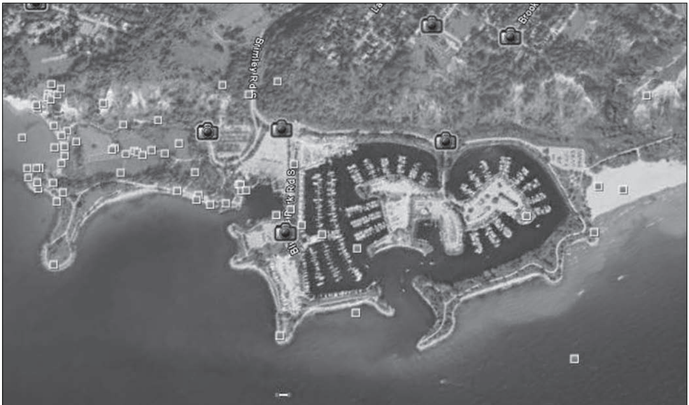
Figure 5. Built on reclaimed land in Lake Ontario east of Toronto, Bluffer's Park first opened in 1975 and was expanded to its current size in the early 1980s. The park is home to four sailing clubs. Note 100-ft scale bar and armored headland on left (Google air photo 2009).
