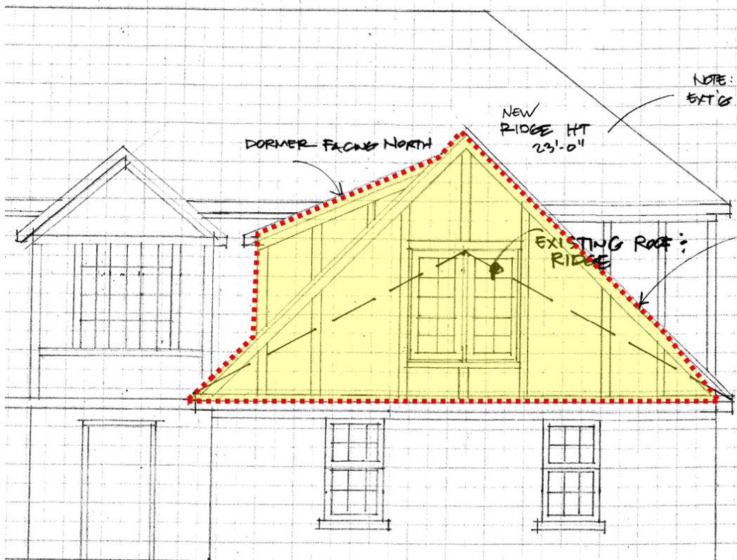
Figure 10 – Amended west elevation of proposed second-floor addition
