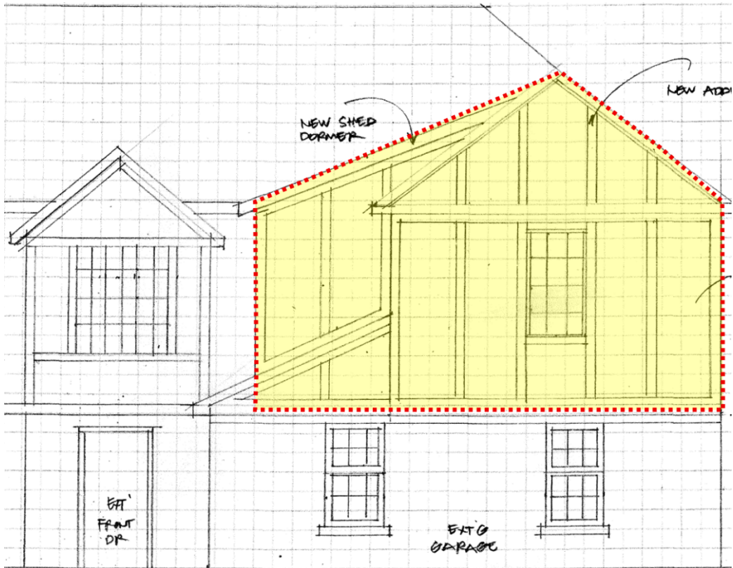
Figure 9 – Previous west elevation of proposed second-floor addition
