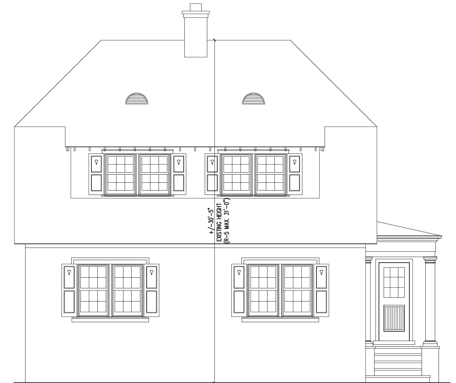
Existing West Elevation 1/4" = 1'-0"
