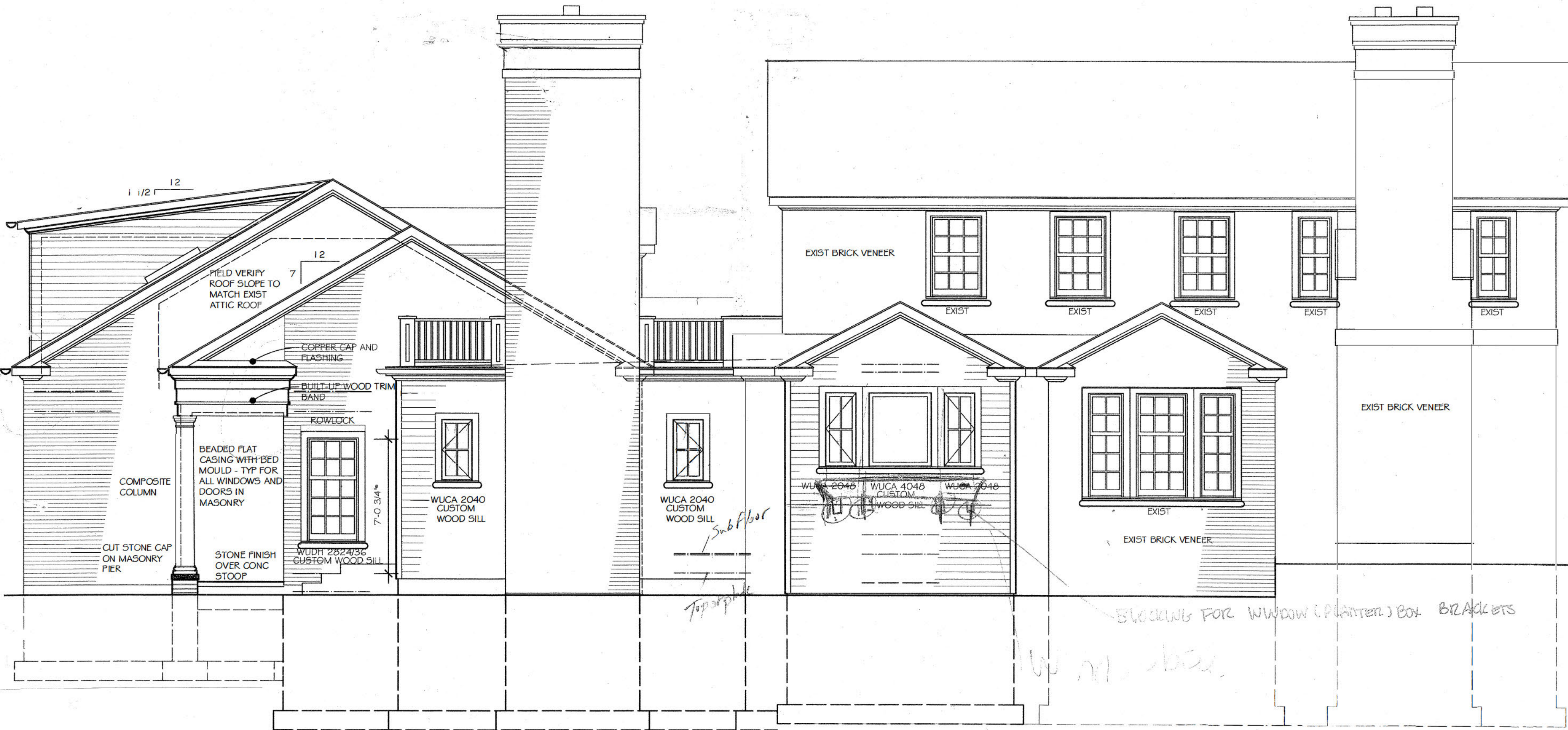
EXISTING WEST ELEVATION 1/4" = 1'-0"
