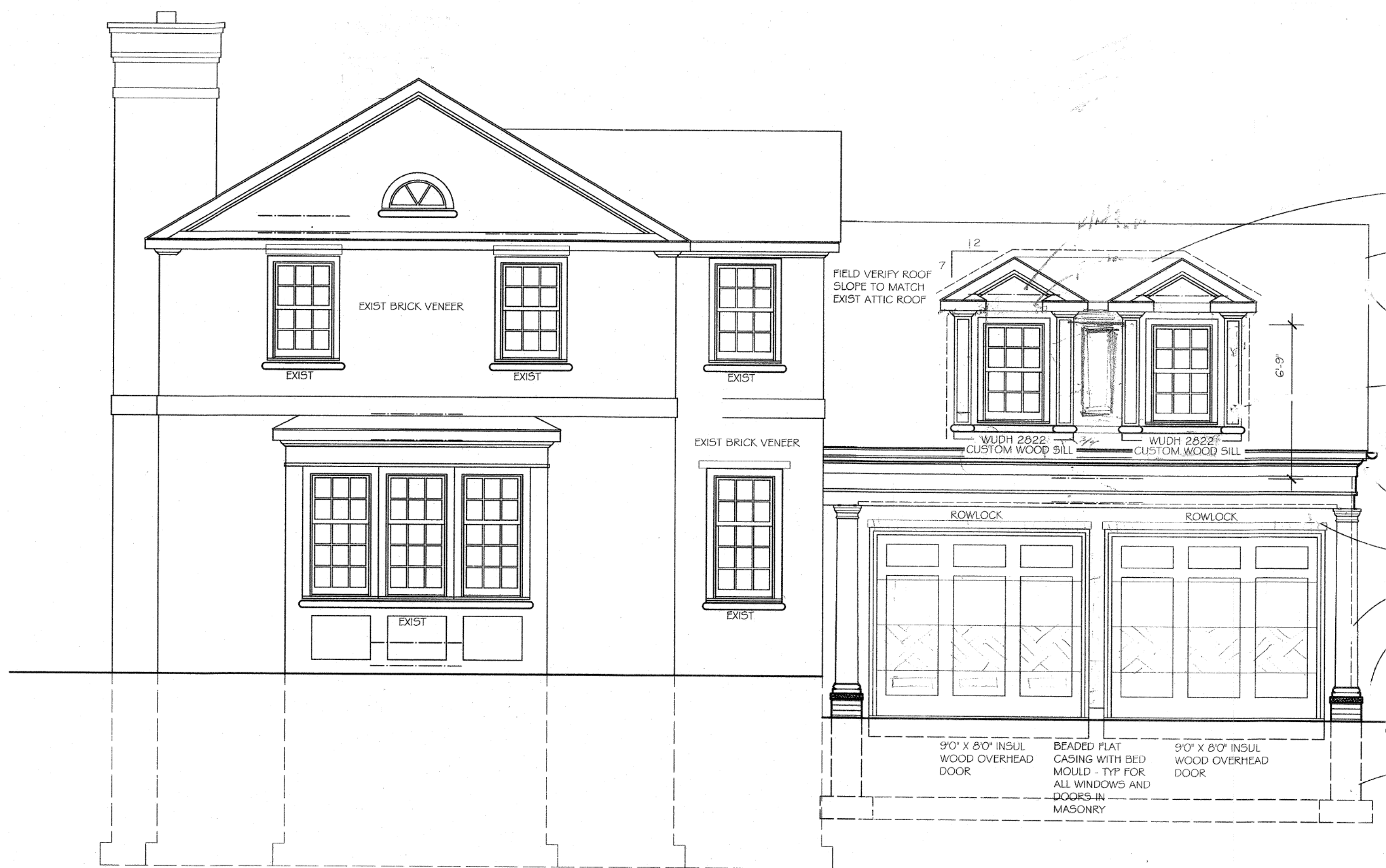
EXISTING SOUTH ELEVATION 1/4" = 1'-0"
