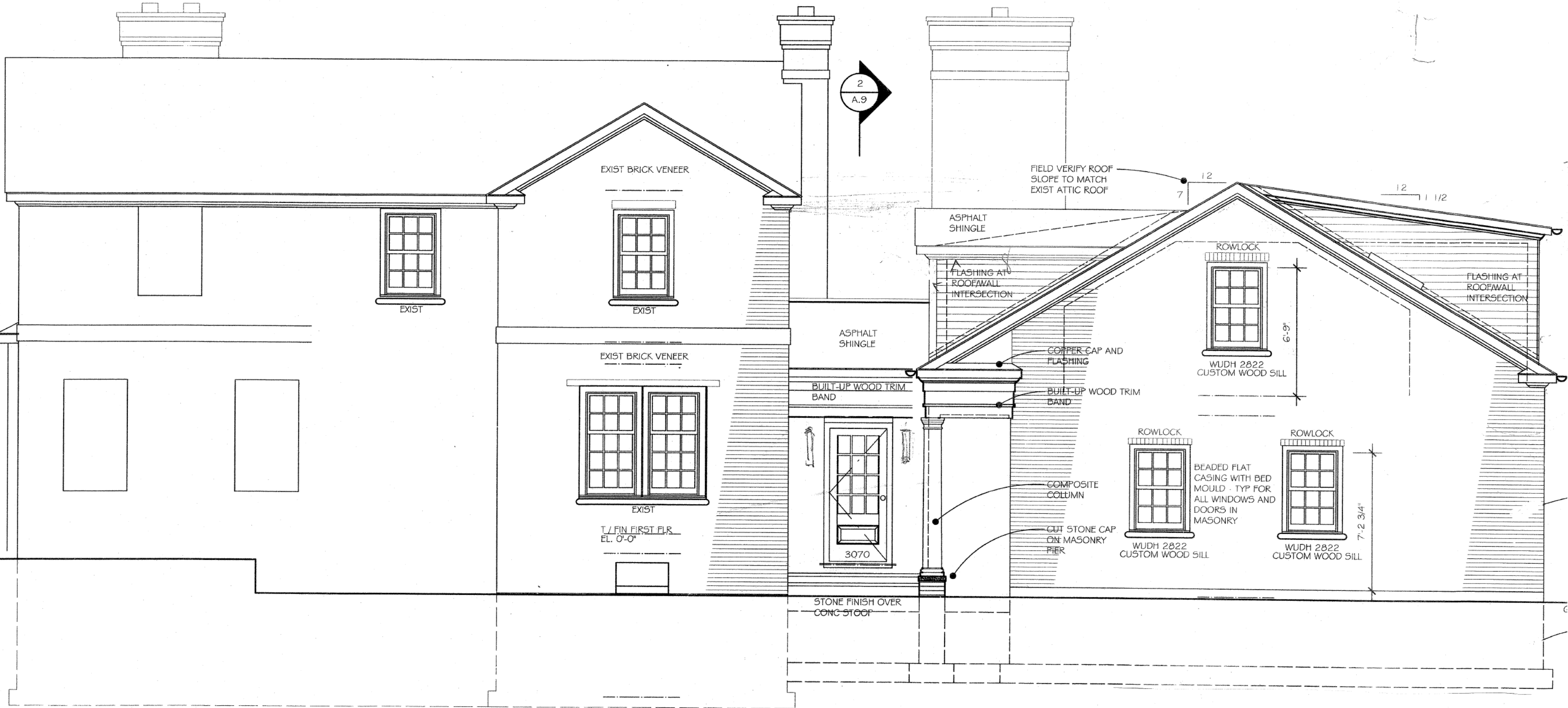
EXISTING EAST ELEVATION 1/4" = 1'-0"
