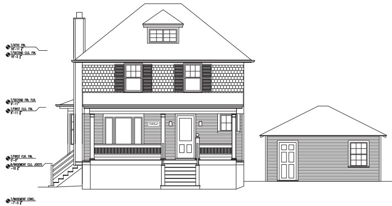
1 Existing Front Elevation East SCALE: 1/8" = 1'-0"
