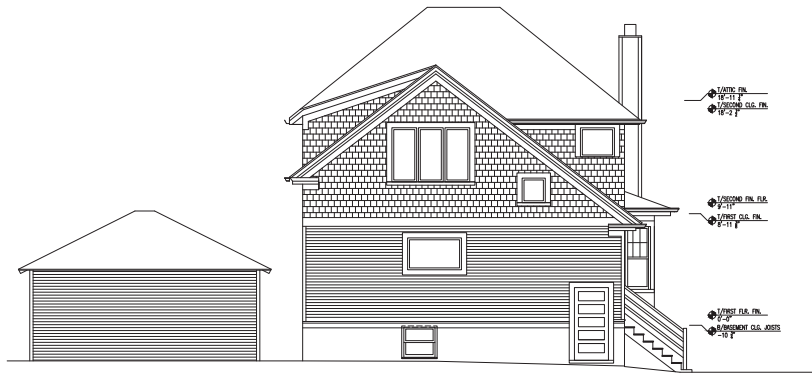
2 Existing Rear Elevation West SCALE: 1/8" = 1'-0"
