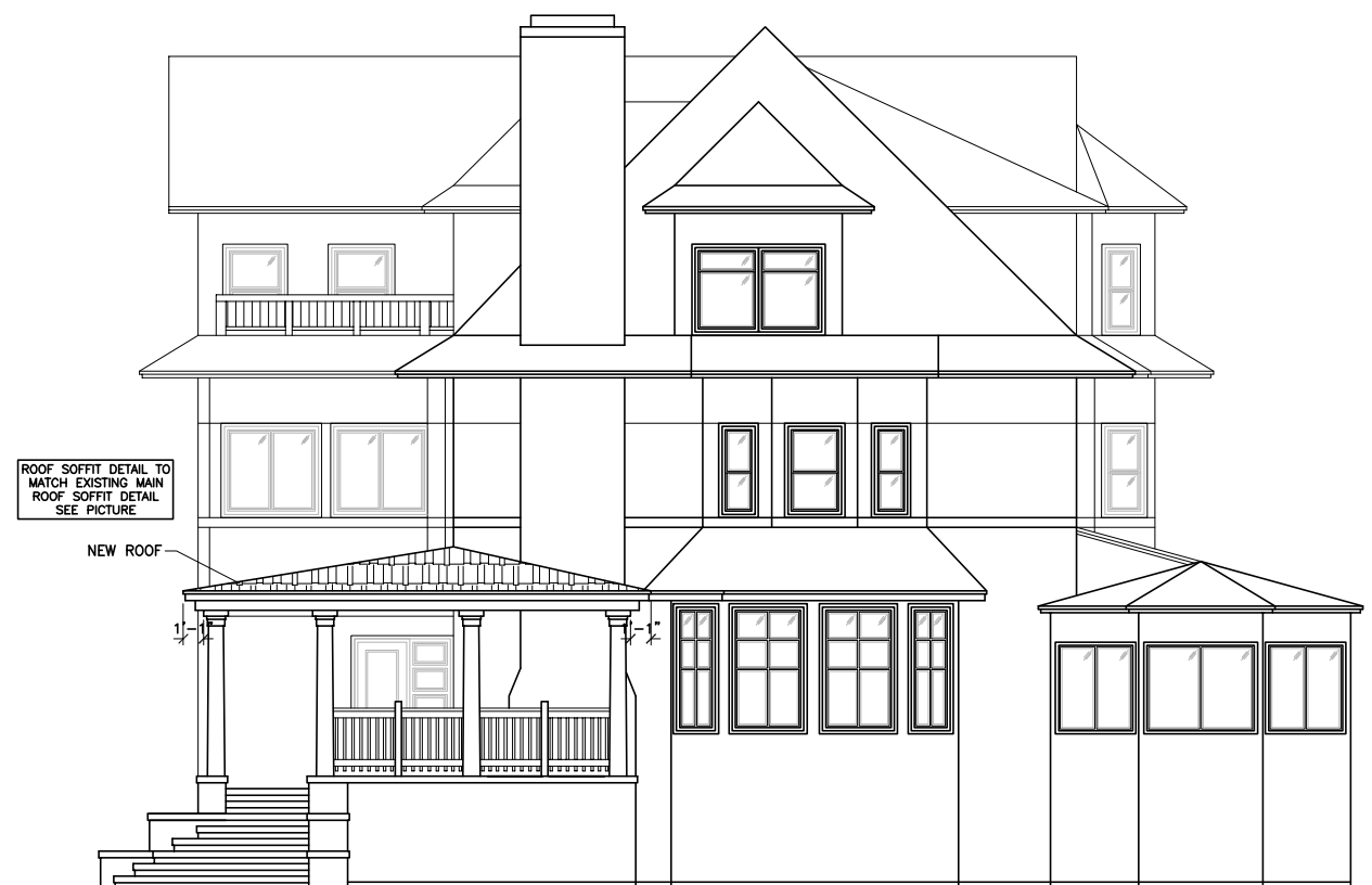
PROPOSED SOUTH ELEVATION SCALE: 3/32"=1'-0"
