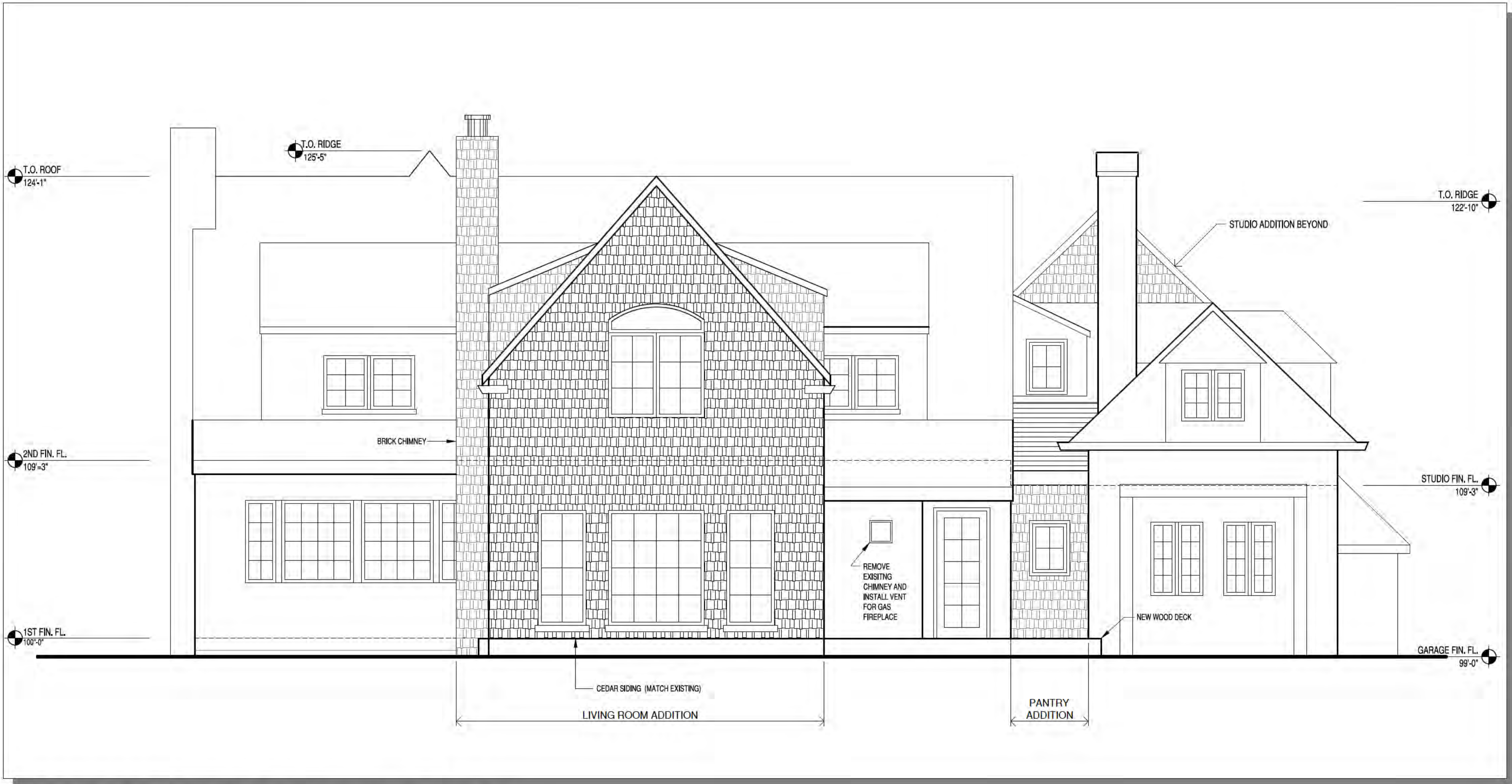
PROPOSED SOUTH (REAR) ELEVATION 1/4" = 1'-0"
