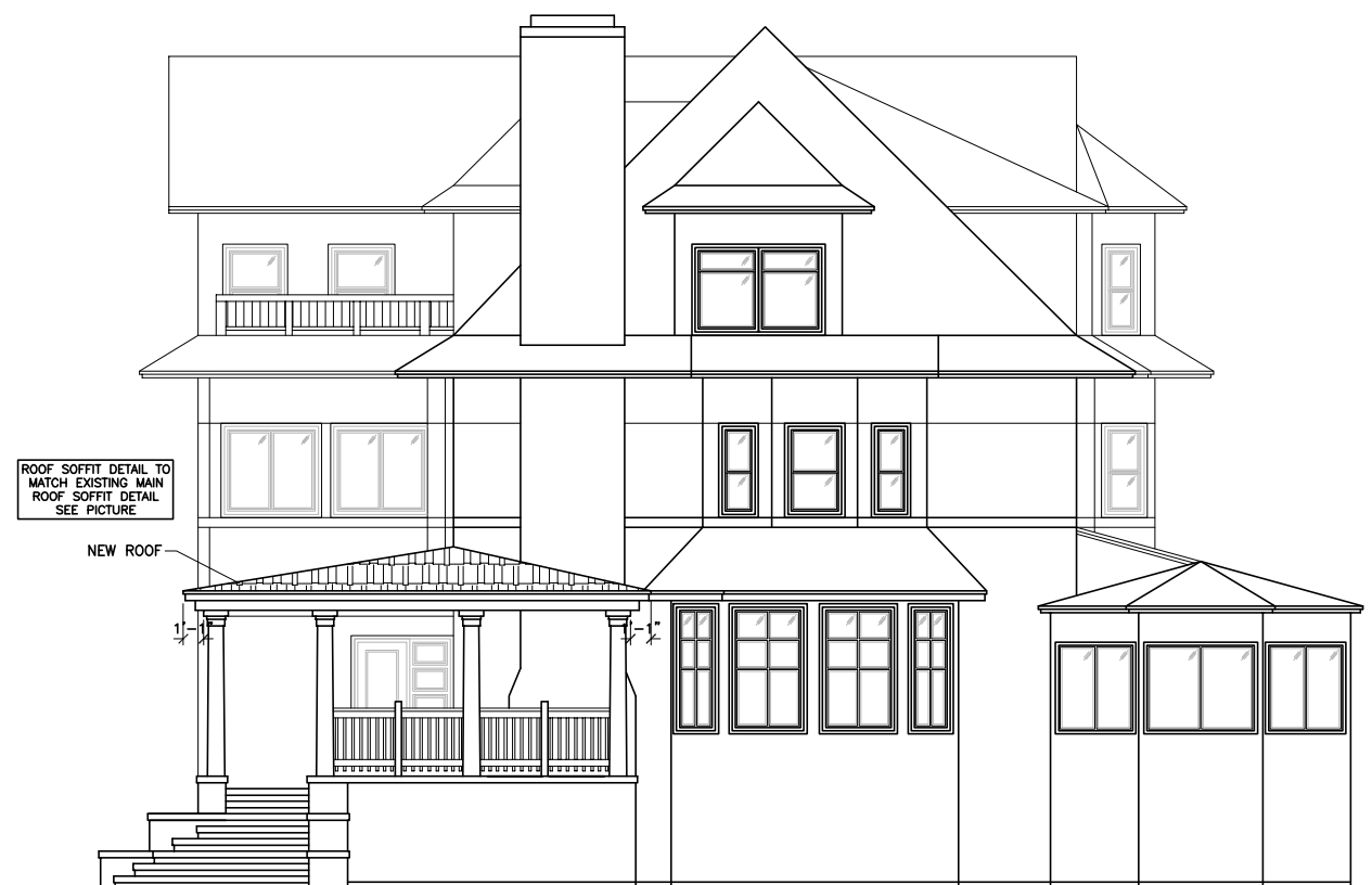
PROPOSED SOUTH ELEVATION SCALE: 3/32"=1'-0"
