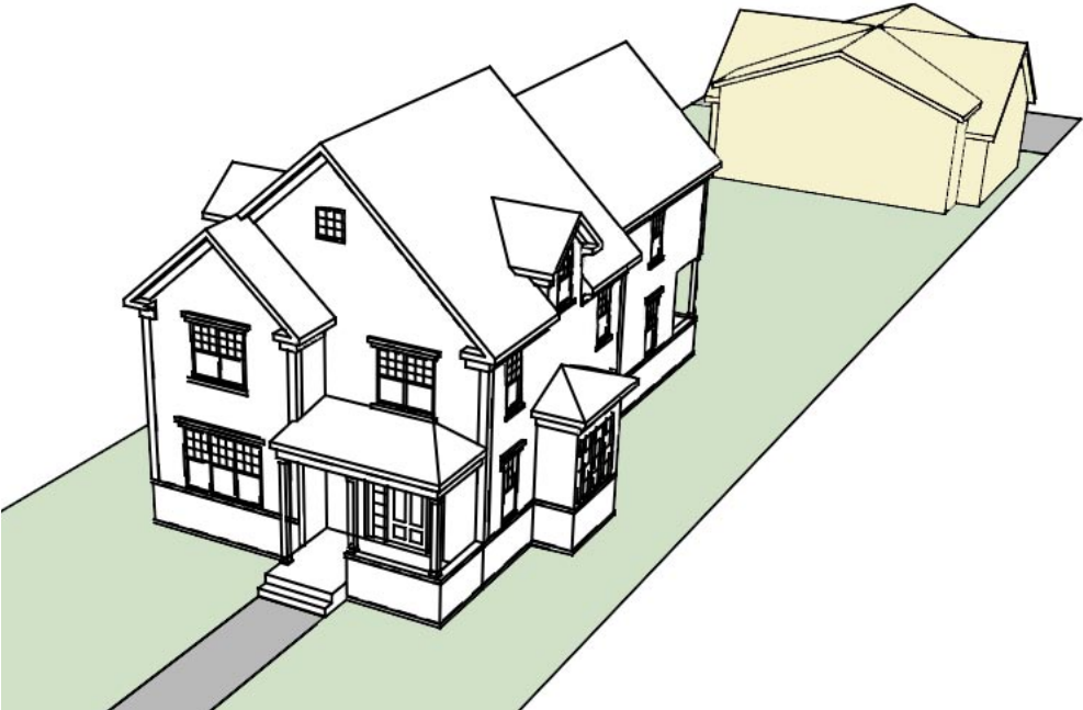
Avoid: The accessory structure appears too large and out of character in comparison to the primary structure.
