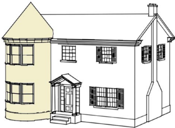
Inappropriate addition of Queen Anne tower to Colonial Revival building.
