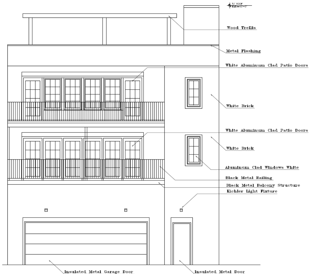
Figure 8 – Rear Building Elevation – Public Alley
