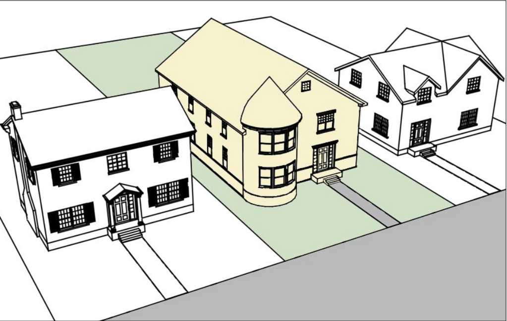
Avoid: Building mass is unbroken, appearing greater in scale than others in the neighborhood.
