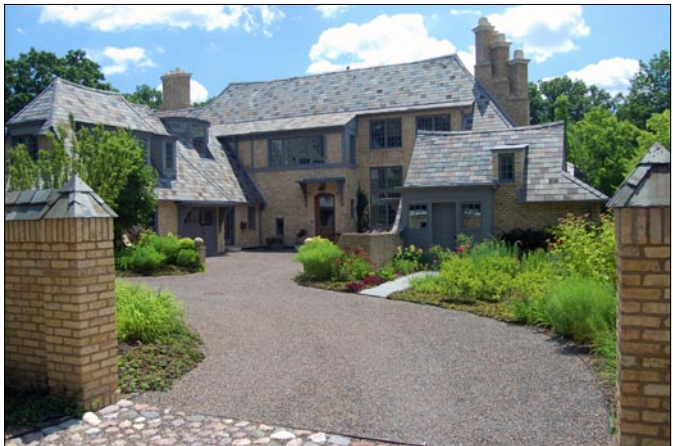
The mass of this larger home is broken into several distinct modules, resulting in attractive facade articulation, and allowing for further reduction of the perceived mass through variations in height and roof form.
